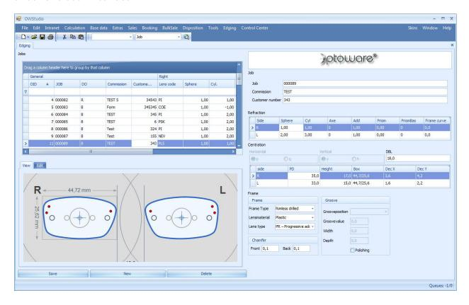
All shape data can be adapted as needed, starting with the size and type all the way to the facet and its measurements as well as the edge thickness requirements for the drill holes. You can also use the shape data perfectly to calculate the lens thickness, for thickness optimization and thus for consultancy purposes.
